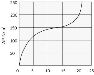
Face Velocity m/sec. (Based on duct area)
